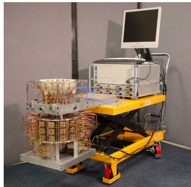
Switching interface (below) between 8 port VNA and antenna array (top)
